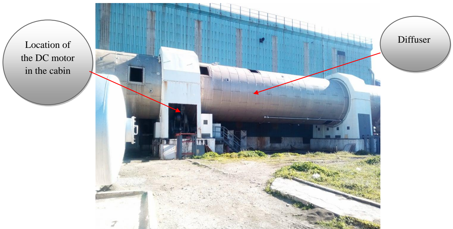
Figure 2 : Diffuser + DC motor
