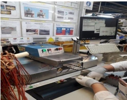
Figure 20: The welding operation
