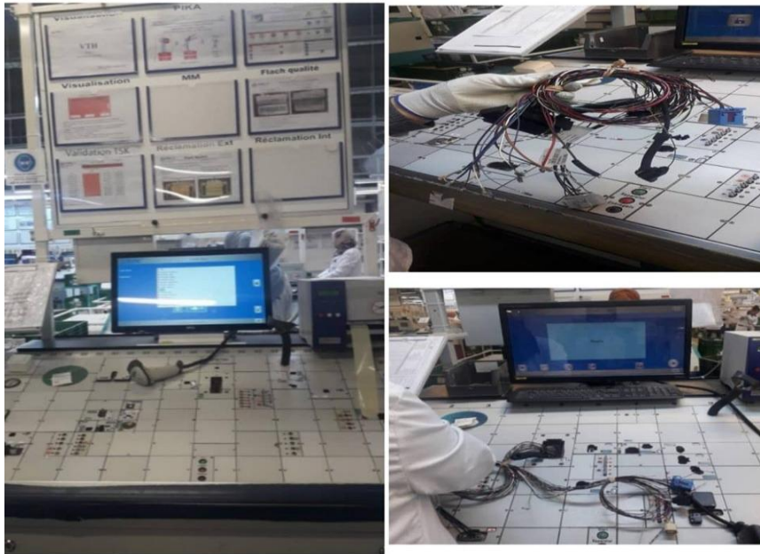
Figure 25: Electrical test table
